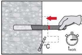
Before use, verify that the steel element is dry and free of oil and other contaminants. Mark and set steel element to the required embedment depth before working time  $t_{work}$  has elapsed. The working time  $t_{work}$  is given in Table B2.
