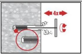
Brush 4 times with the specified brush (see Table B3) by inserting the steel brush Hilti HIT-RB to the back of the hole (if needed with extension) in a twisting motion and removing it. The brush must produce natural resistance as it enters the drill hole (brush  $\phi \geq$  drill hole  $\phi$ ) - if not the brush is too small and must be replaced with the proper brush diameter.
