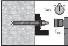
After required curing time  $t_{cure}$  (see Table B2) the fastening can be loaded. The applied installation torque shall not exceed the values max.  $T_{inst}$  given in Table B1.
