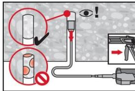
Overhead installation and/or installation with embedment depth  $h_{ef} > 250$  mm.
