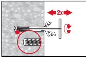
Brush 2 times with the specified brush (see Table B3) by inserting the steel brush Hilti HIT-RB to the back of the hole (if needed with extension) in a twisting motion and removing it.
