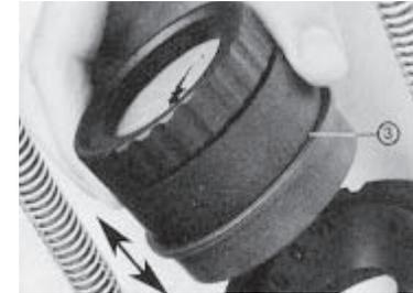
Insert the water collector (3) and press it down firmly into the holder. Connect the water extraction hose.
