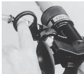
The water supply valve can be regulated using the index finger.
