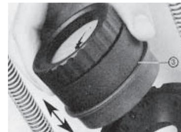
Insert the water collector (3) and press it down firmly into the holder. Connect the water extraction hose.
