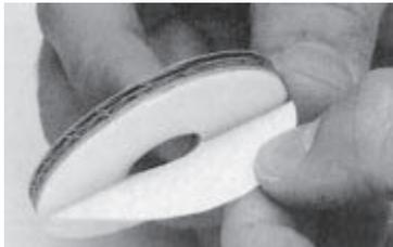
Hole-starting aid for dry drilling: Use the appropriate disc for each core bit diameter. Apply the self-adhesive disc where the hole is to be drilled after removing the protective foil. Nails can be used if the adhesive is not effective. The self-adhesive centering disc can be used only once.
