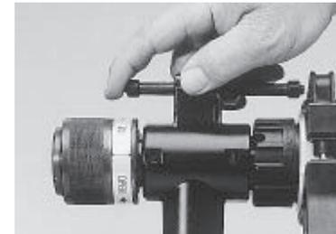
Push the chuck rotation-prevention pin into the opening provided.
