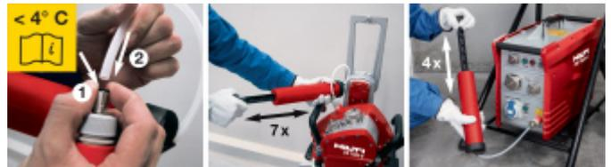
Removing cooling water from the saw head and power supply
