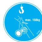
The saw head and accessory transport trolleys may be lifted by crane only at the lifting points provided.
