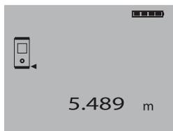
If further measurements are taken, up to three previously determined distances are shown in the intermediate result lines, i.e. a total of the last four measured distances are shown.
