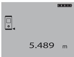
You have taken the first distance measurement with the PD 30 range meter.
