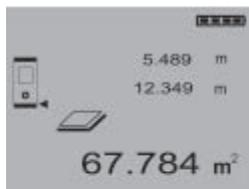
Both distances required to calculate the area appear in the intermediate result lines and can be conveniently noted after the measurements and the calculation.
