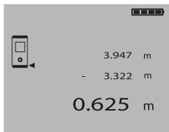
This procedure can be followed until all distances have been subtracted. To terminate the subtraction of distances, simply measure a distance without first pressing the "Minus" key. The previous measurement and calculation results will be shown in the intermediate displays.
