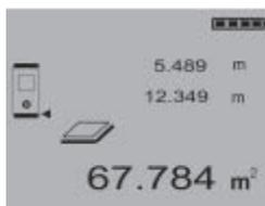
Both distances required to calculate the area appear in the intermediate result lines and can be conveniently noted after the measurements and the calculation.
