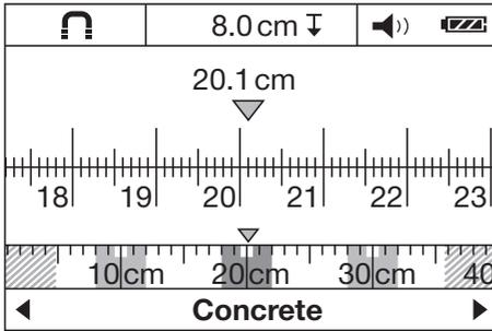
The display mode can be changed in all scanning modes. This function changes only the display mode, not the scanning mode.
