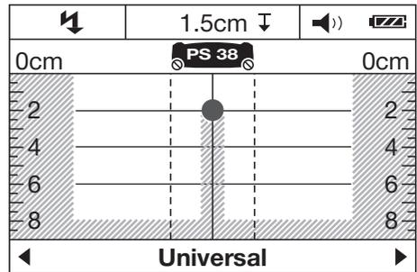
A live metallic object, e.g. an electric cable, is within the sensor area. It lies at a depth of approx. 1.5 cm (0.6 in). The tool emits a warning signal tone for “live cables” as soon as the electric cable is detected by the sensor.
