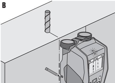
1. A single scan of the area is sufficient for initial location of an object.
