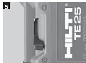
**Note:** A major feature is the infinitely variable speed switch for the RPM and hammering speed
