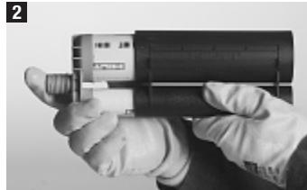
Insert the foil pack (7) into the holder (6) as far as it will go and then screw on the mixing nozzle (8 or 9).
