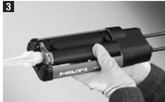
Before inserting the holder in the dispenser, the piston advance rods (1) must be pulled into the rearmost position while pressing the release lever (2). See photo 8.
