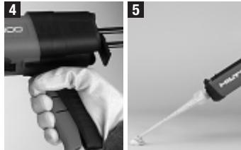
Pull the trigger (4). The foil pack is opened automatically by a piercing point built into the junction piece. The 2 components can be seen to mix as they pass through the nozzle.
