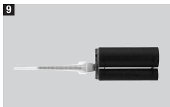
Partly used foil packs should be stored in the holder with the mixing nozzle screwed on. The adhesive mortar in the mixing nozzle will become hard during a long pause.
