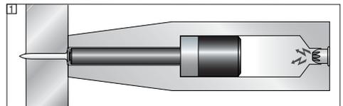
The energy from the propellant charge is transferred to a piston, the accelerated mass of which drives the fastener into the base material. As approximately 95 % of the kinetic energy is absorbed by the piston, the fastener is driven into the base material at much reduced velocity (less than 100 m/sec.) in a controlled manner. The driving process ends when the piston reaches the end of its travel. This makes dangerous through-shots virtually impossible when the tool is used correctly.
