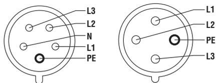
L1 = fase 1, L2 = fase 2, L3 = fase 3, N = conductor neutro, PE = masa / tierra
