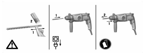
Fit the accessory tool into the SDS chuck or, respectively, remove the accessory tool from the SDS chuck.
