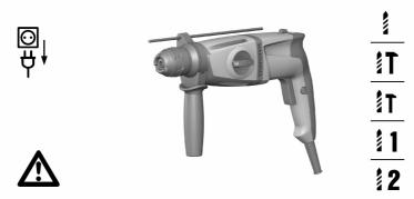
Set the function selector switch to the "Drilling with hammering action" (hammer drilling) position ?T.
