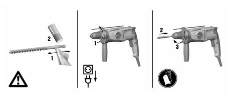
Fit the drill bit or other accessory in the quick-release chuck or, respectively, remove the drill bit or other accessory from the quick-release chuck.
