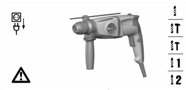
► Set the function selector switch to the "Drilling" 💈 position.
