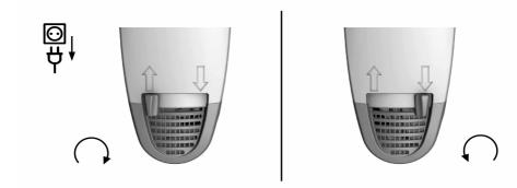
Set the forward / reverse selector switch to forward or reverse rotation.
