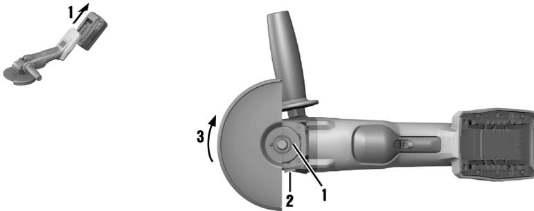
1. Fit the guard onto the drive spindle collar so that the two triangular marks on the guard and on the power tool are in alignment.
