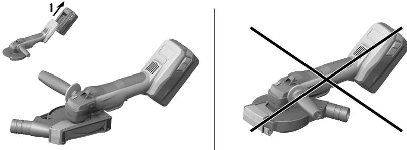
1. Position the front cover with the closed side on the standard guard and push it on until it engages.
