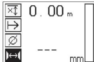
The correct diameter must be known and previously entered. The bar spacing distance must also be entered if within the  $36 \text{ mm} \leq s \leq 120 \text{ mm}$  ( $1.41'' \leq s \leq 4.72''$ ) range. This value can be taken from building plans, confirmed by chipping away a channel in the concrete to view the bars, or measured using Quickscan detection.
