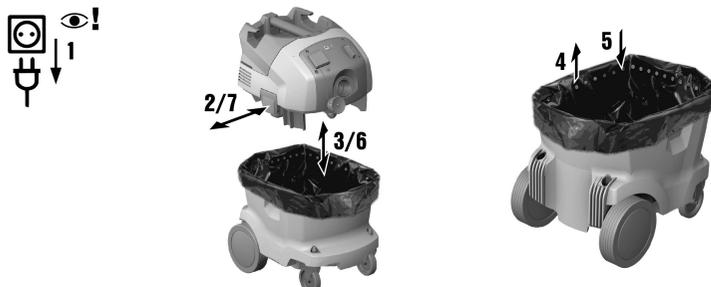
1. Disconnect the supply cord plug from the power outlet.
