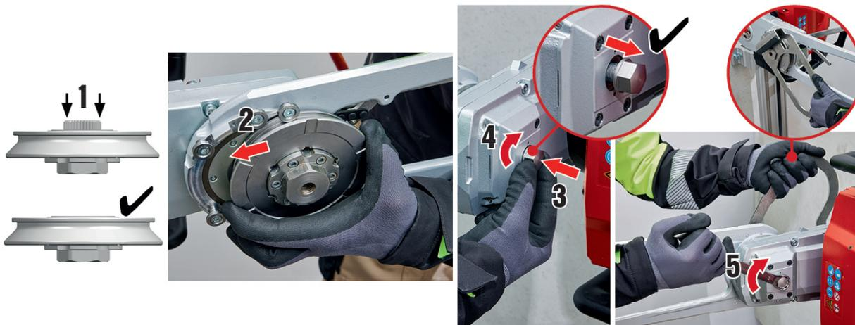
2. Press the flange nut fully into the inner flange **(1)**.
