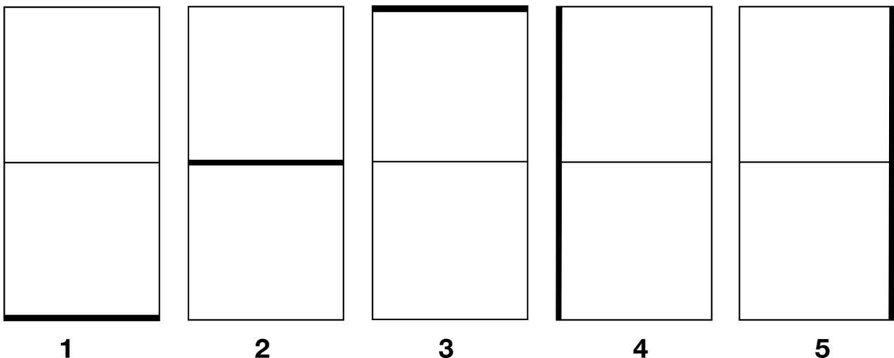
The illustration shows an example of the cutting sequence for a door opening with a dividing cut
