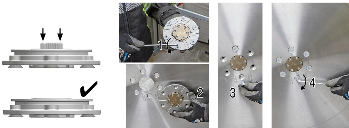
2. Press the flange nut fully into the inner flange.
