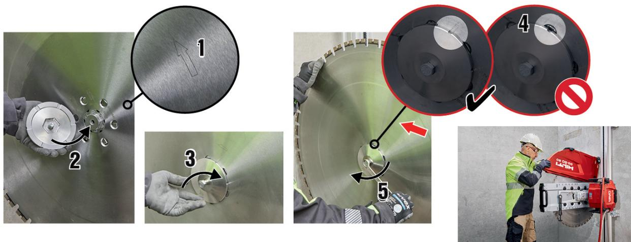
1. Fit the saw blade on to the centering device on the flange.
