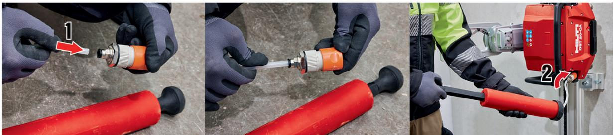
1. Push the pump hose on to the blow-out adapter as far as it will go **(1)**.
