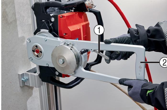
① Lever, keyless locking system                      ② Blade guard holder
